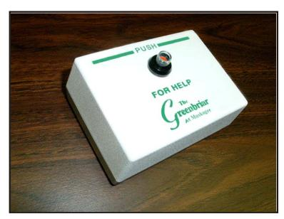
The TTS-01wireless emergency call switch is shown here with custom printing. The pushbutton switch latches in the alarm position when it is pushed and displays an orange alarm status indicator in the top of the button. When the care giver pushes the button again, the orange indicator disappears and the switch initiates a restoral transmission.
